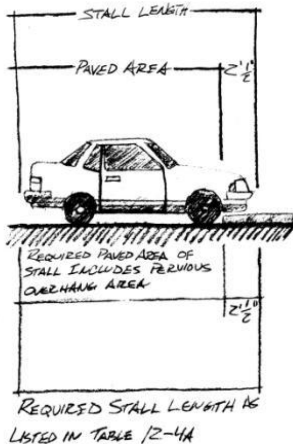
FIGURE 12-4D PAVEMENT AREA ADJUSTMENT WITH CONTINUOUS CURB USAGE
