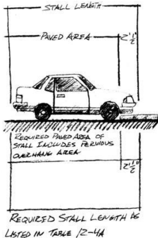
FIGURE 12-4D PAVEMENT AREA ADJUSTMENT WITH CONTINUOUS CURB USAGE
