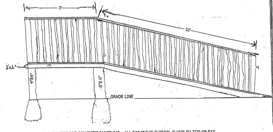
NOTE:...ALL SUPPORT CONCRETE 31" TO 34" ALL RAILING IS 3' FROM FLOOR TO TOP OF RAIL. ALL RAILS ARE 2"X2" X3'.
