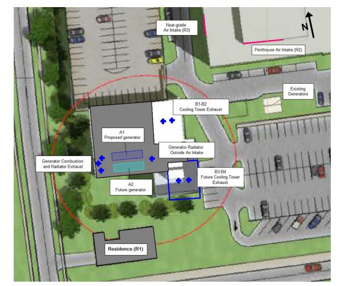
Figure 1: Plan Sketch of Equipment Layout for New Energy Plant
