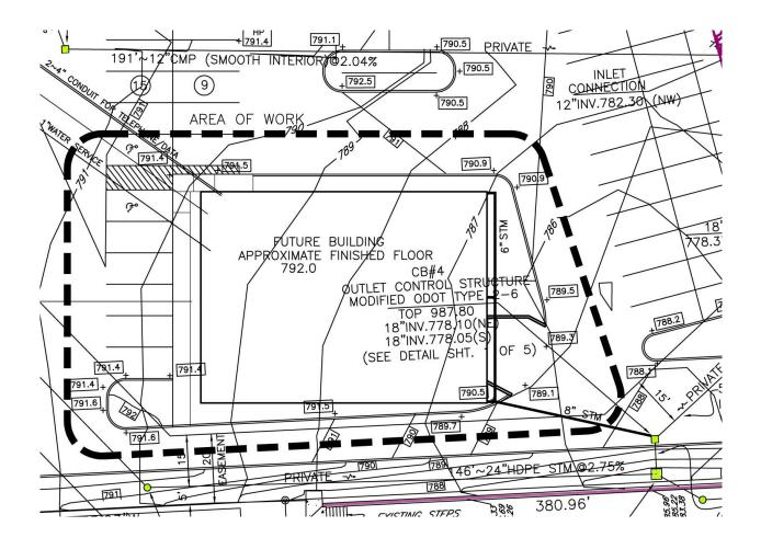
Copies of minor adjustments to the existing curbs and establishment of the proposed building finished floor are being provided. These are all minor adjustments to the overall site as it was originally designed to accept a building of this size.
