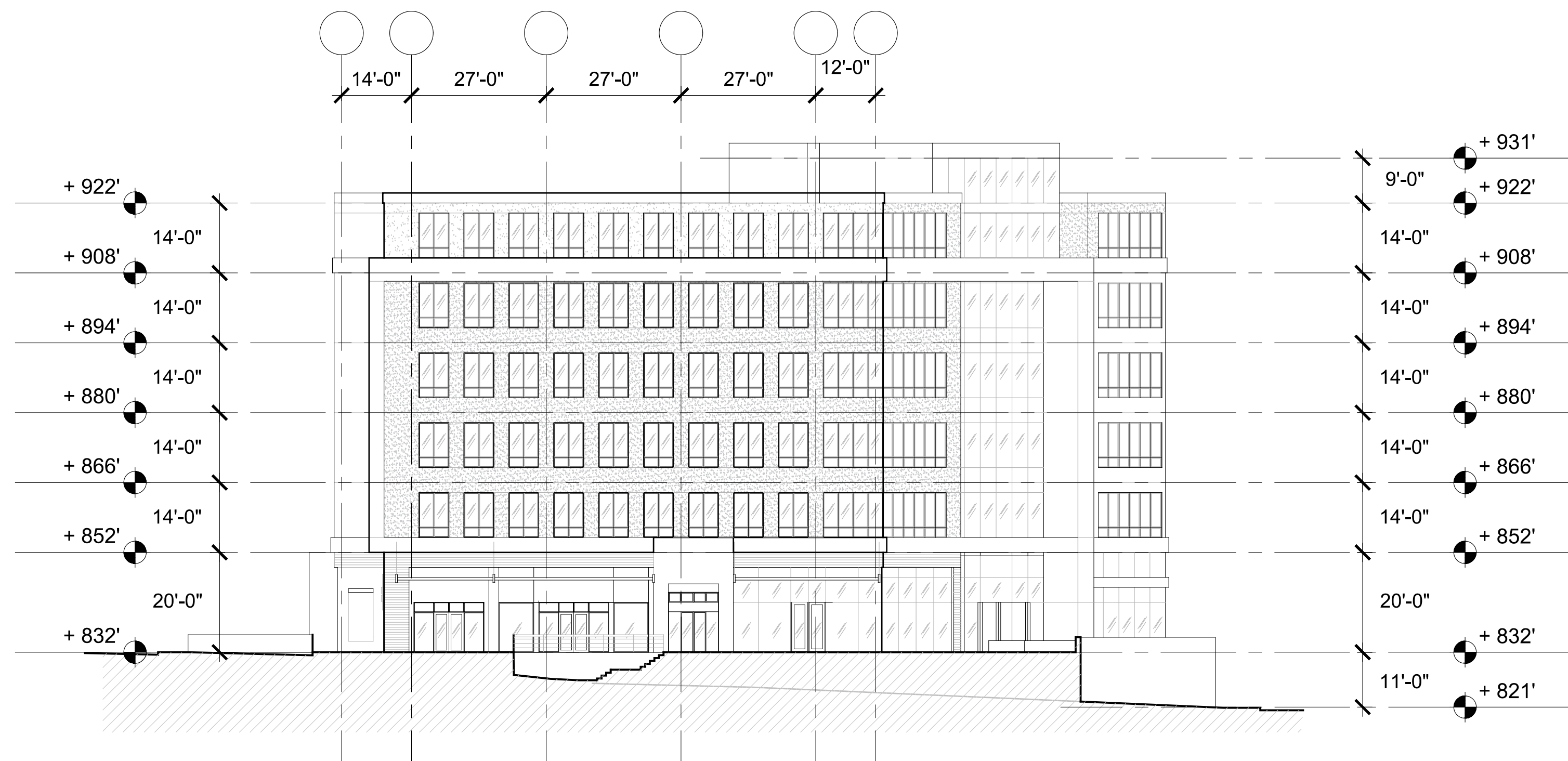
1 OFFICE BUILDING EAST ELEVATION 1"=20'
