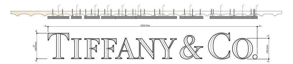
LED Metal Channel R3D Sign Scale: 1/1 Fluted Stone Wall AC-DC Power Supply Body: Stainless-steel Channel Brushed Finish 6mm Frame Fuse Box AC100-240V <u>Light Source:</u> SMD-LED (White) on Custom Designed Circuit Board Cable Cover (Matte White) L=40mm Connector \*Total Cable Length: 10m Face: Clear Acrylic 5mm Thick Frosted Ridge + Reverse 3D Effect Finish M4 Stud bolt w/ Acrylic Spacer (Matte White)
