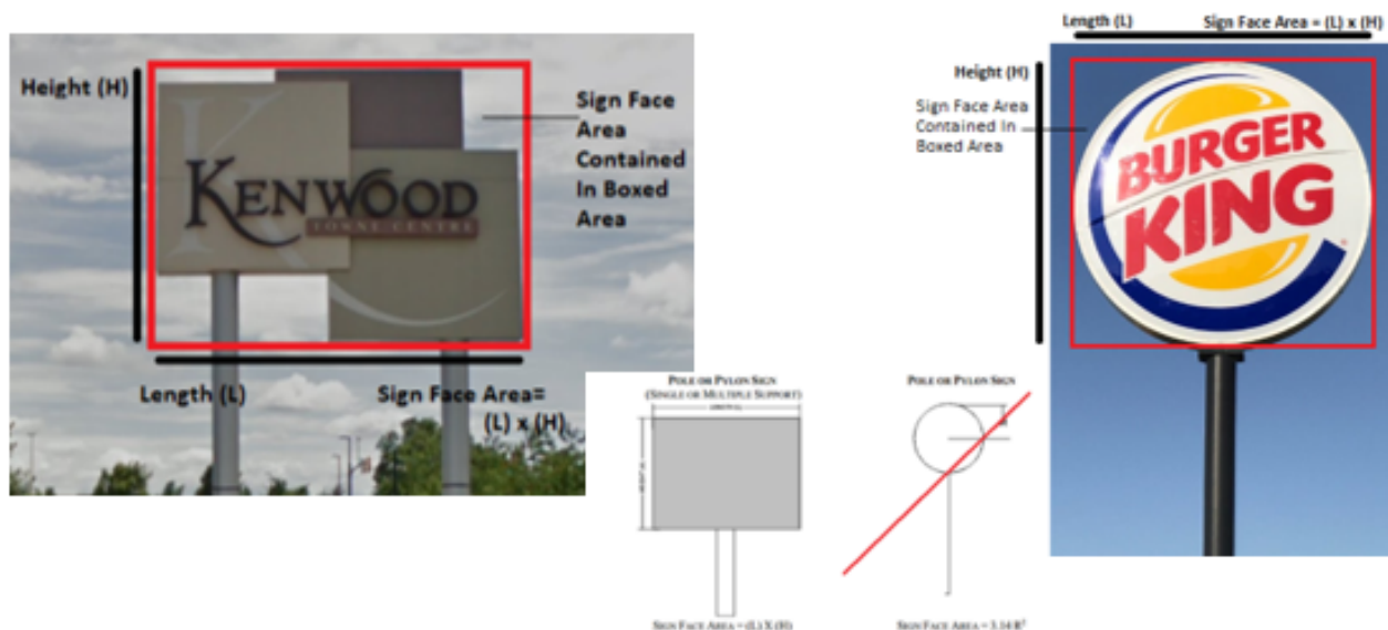
FIGURE 13-6A: SIGN FACE AREA MEASUREMENT POLE OR PYLON SIGN
